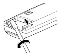
3. Insert the flathead screwdriver into the gap between the cover and the transmitter, and then rotate the screwdriver to detach the cover.
